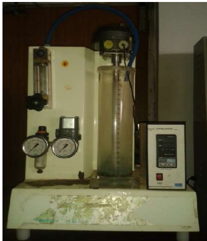
Figure 3 . Level Process Setup
